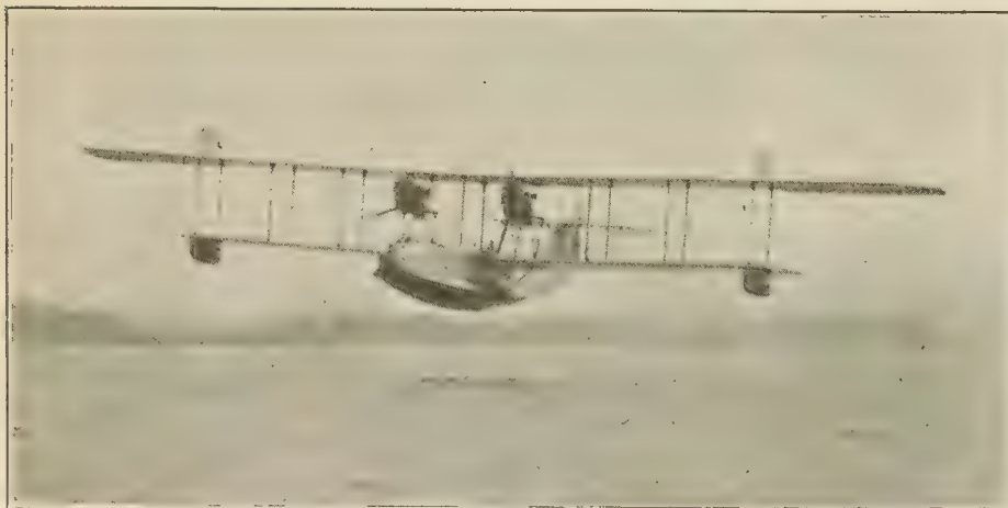
F-5-L—Flying Boat—Front View in Flight, Close to Water Equipped with 2 Liberty-12; 107 ft. span; 50 ft. long; 102 m. p. h. maximum speed; weight, fully loaded, 14,000 lb.; crew, 4-5 men; radio apparatus
